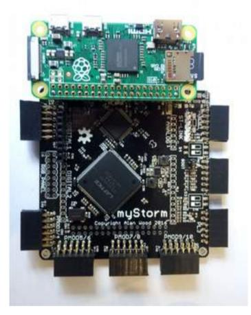
MyStorm is a brand new \$30 open source hardware platform designed to allow the exploration of new processor architectures.
